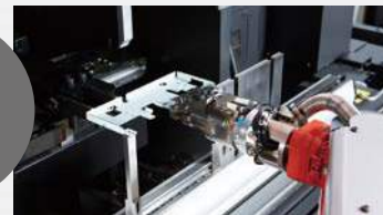
Cut sheets are bent into desired shapes
